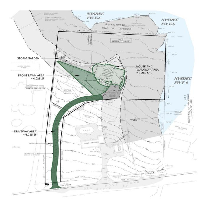
The following figures, Figures 2 through 3 represent the runoff values produced for the portions of the property that are anticipated to be new impervious surfaces, both in the pre and post developed condition for a 6.38"/24-hour Type III (25 Year Storm) rainfall event tributary to the storm garden.
