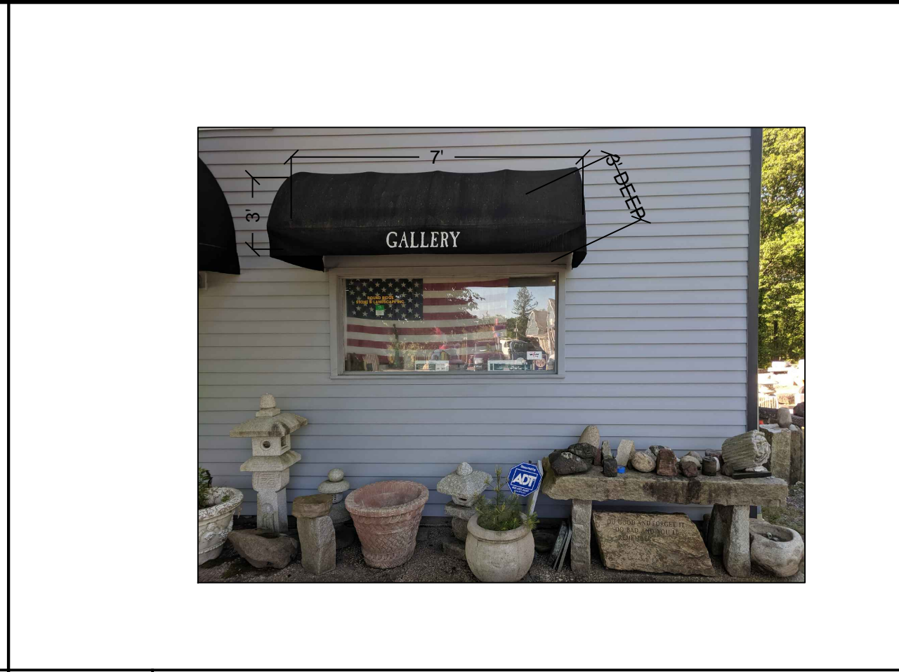
SN-3 FRONT WINDOW CANOPY SIGN DETAIL NOT TO SCALE
