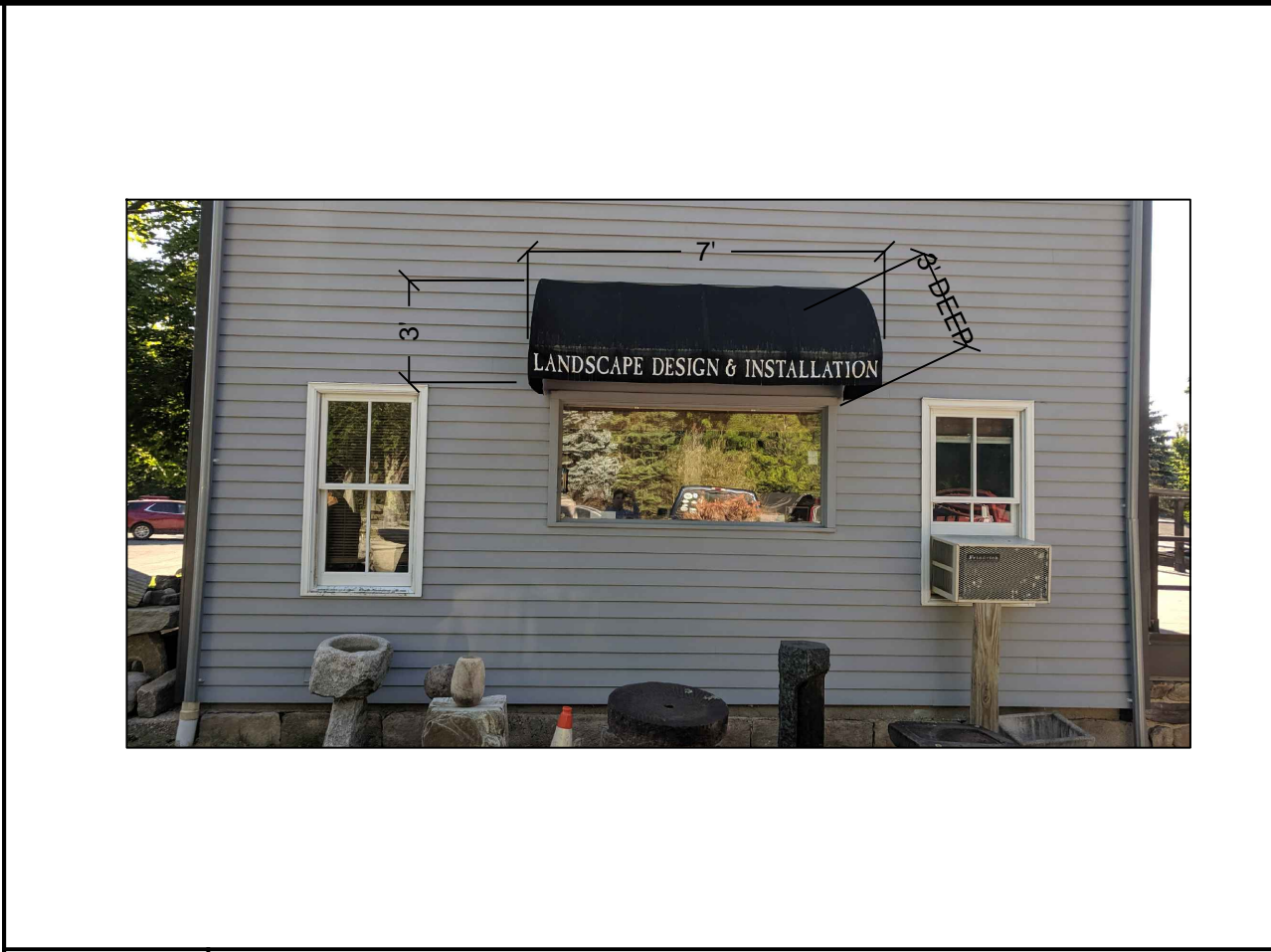
SN-2 EAST SIDE CANOPY SIGN DETAIL NOT TO SCALE
