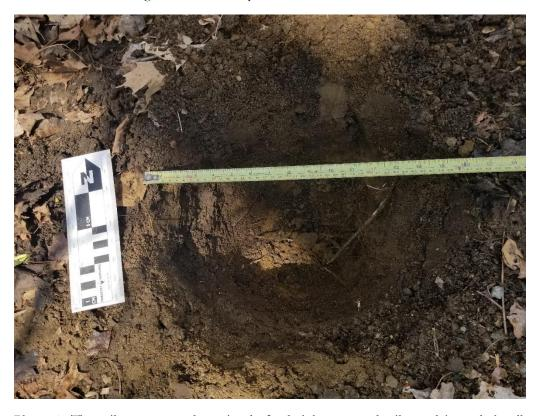
Photo 6: The soils encountered consisted of a dark brown sandy silt overlying a dark yellow brown silty sand with gravel. View of STP 4.
